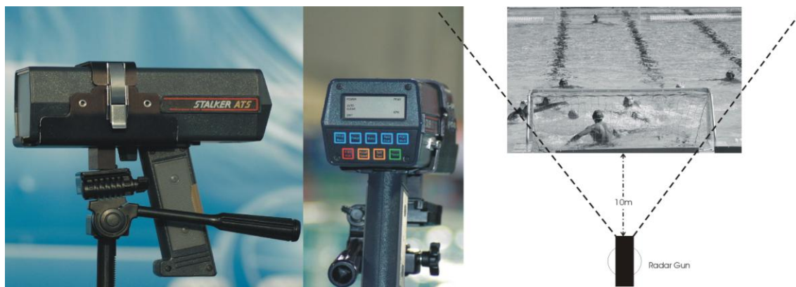
Figure 1. A Schematic representation of the radar position with a model radar gun (StalkerPro Inc., Plano).
