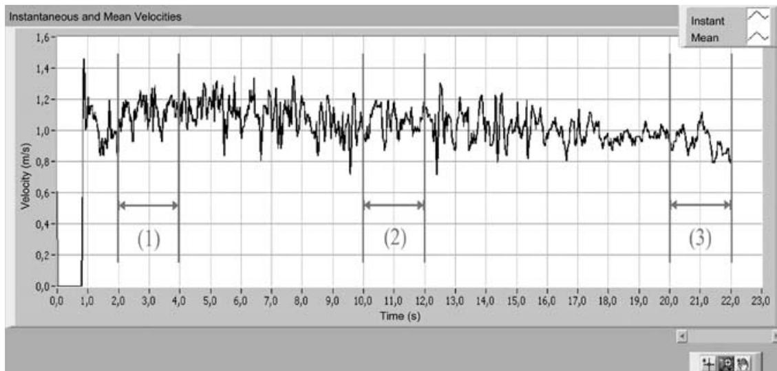
**Figure 6** — Instantaneous velocity curve,  $v(t)$ , obtained using the velocimetric system and time intervals used to calculate mean initial (1), half (2), and final (3) velocities.
